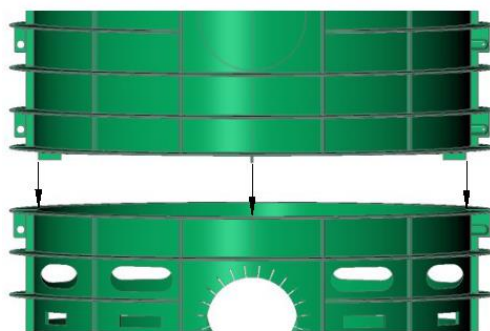
ALIGNMENT TABS FIT INSIDE LOWER FDU
