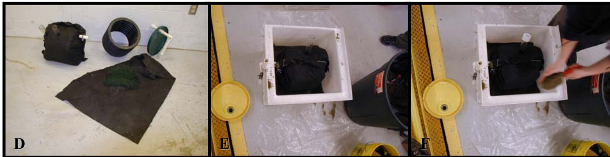
Figure 2. Assembly of the model leaching systems used in the UNH research project. A) An 8" length of distribution line is surrounded by a cubic foot of washed stone atop 3" of washed concrete sand in a square container. B) The stone is surrounded by sand. C) A piece of fabric prevented sand from falling into the spaces between the stones. D) The components of the 12" length of Enviro-Septic ® pipe and how they were assembled. The clear tubes were put in place to enable viewing the inside of the system. E) The Enviro-Septic ® pipe was placed atop 3" of washed concrete sand in a square container and F) surrounded by sand.
