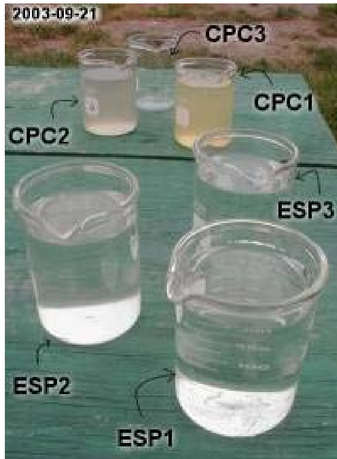
Figure 6. Photograph showing leachate samples from the three different sections of each model leaching system in Stoke, Quebec. The leachate coming out of the Enviro-Septic ® system looks clear to the naked eye, whereas the leachate exiting the conventional pipe and stone system is brown in color and cloudy. The beaker labeled CPC 3 is empty because STE had not reached the third 20' section of the conventional system at the time this photograph was taken.
